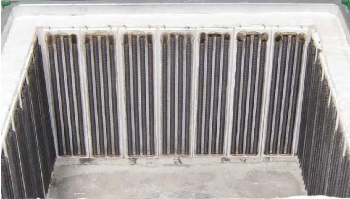
**RAYTEQ MELTING FURNACE EQUIPPED WITH VERTICALLY MOUNTED, PARALLEL-WIRED IRON-CHROME-ALUMINUM (ICA) HEATING ELEMENTS**
