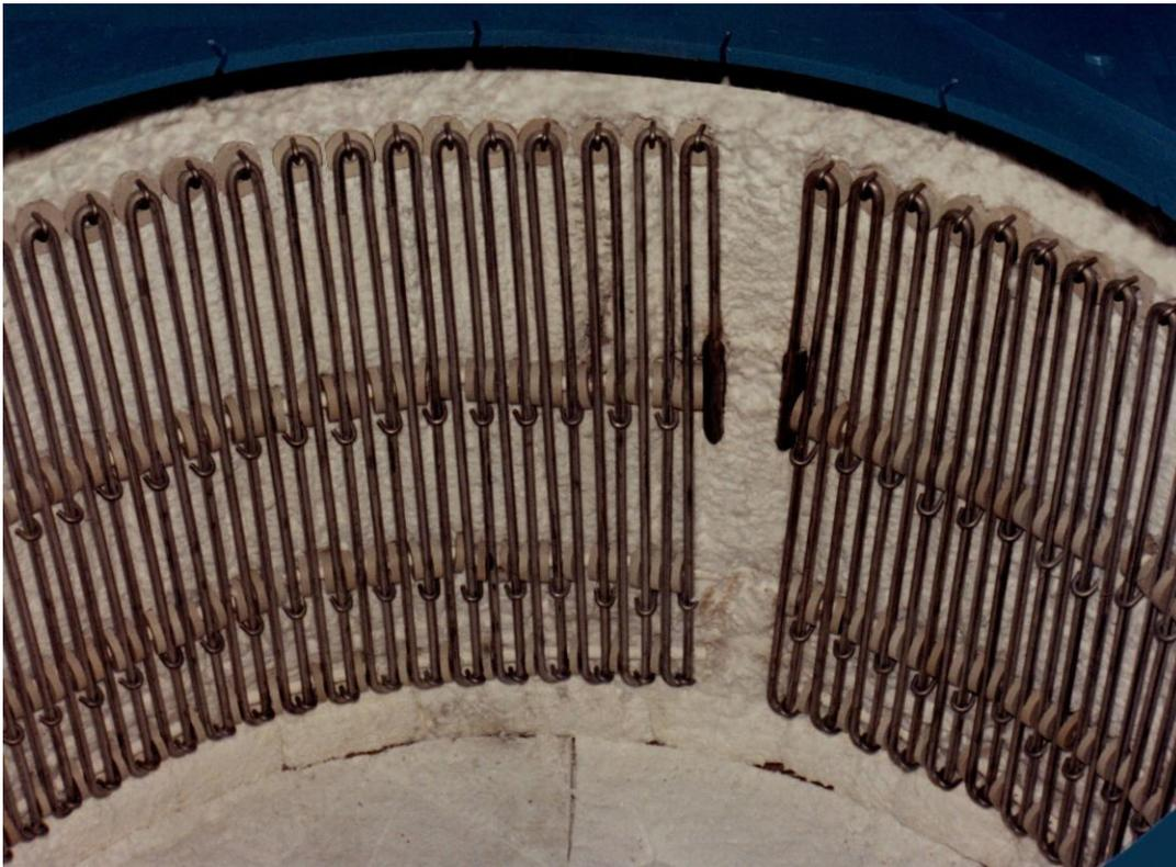
**ROD-OVERBEND STYLE SERIES-CONNECTED NICKEL-CHROME HEATING ELEMENTS IN ELECTRIC RESISTANCE MELTING FURNACE**
