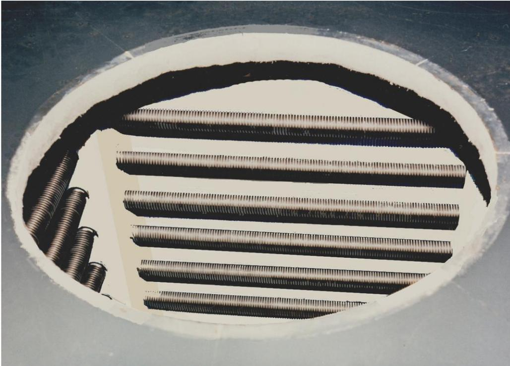
**ELECTRIC MELTING FURNACE EQUIPPED WITH SIX HORIZONTAL COILS OF SERIES-CONNECTED NICKEL-CHROME HEATING ELEMENTS**
