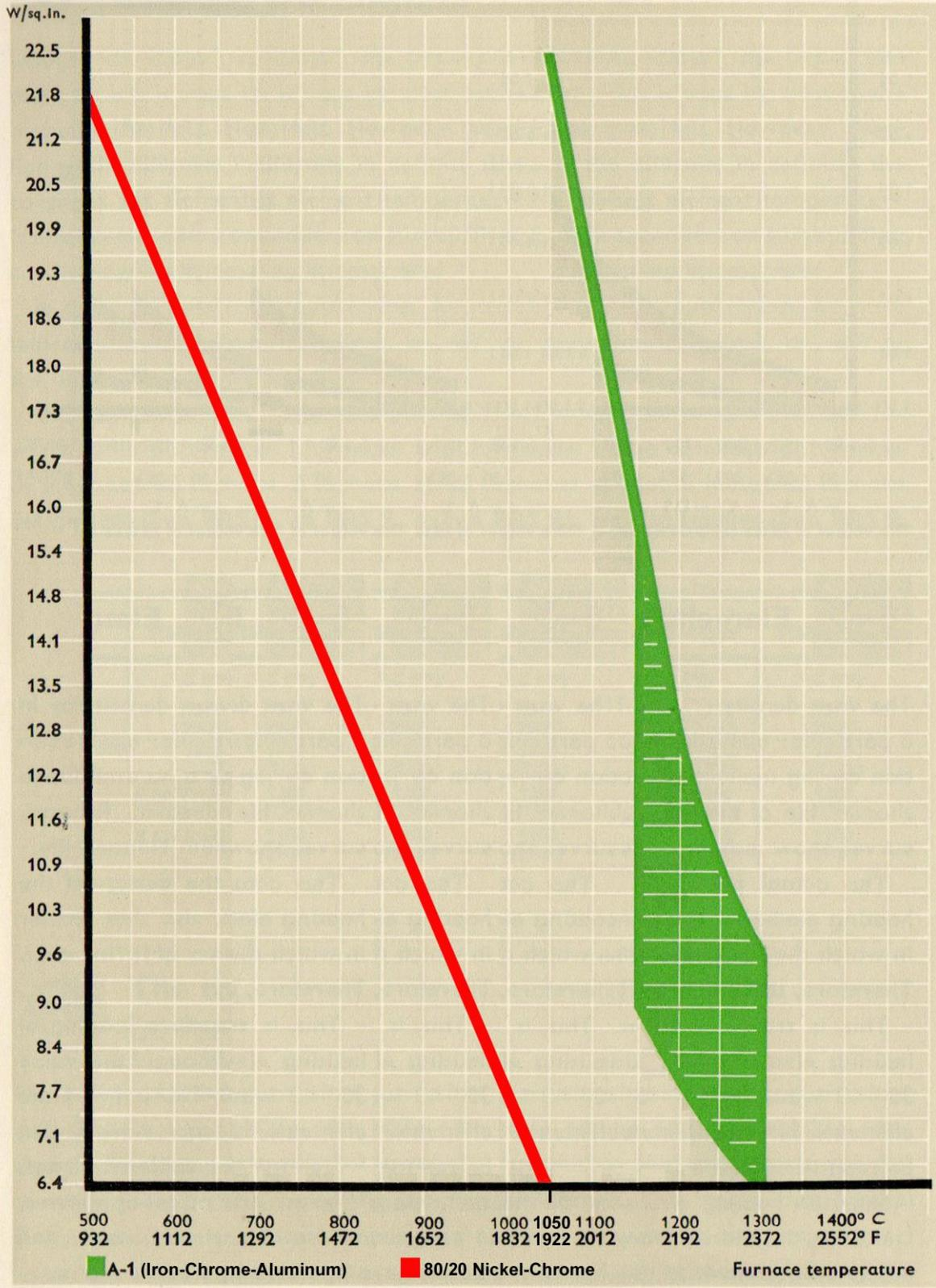
Inconel, etc. The green curve is for iron-chrome-aluminum (ICA) alloy used by Rayteq. Each curve plots maximum recommended watt-density vs. furnace temperature and also shows the recommended temperature limit for both. For easy comparison purposes, the red nickel-chrome alloy curve has been superimposed on the ICA graph.
