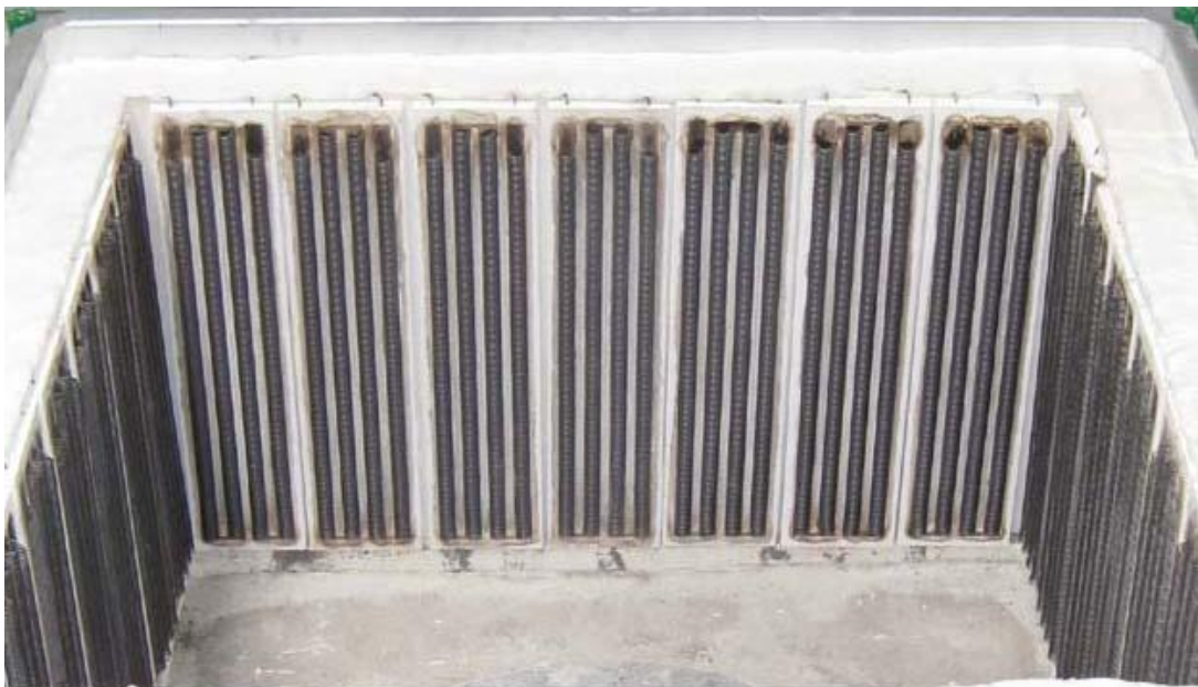
RAYTEQ MELTING FURNACE WITH PARALLEL-WIRED HEATING ELEMENTS
